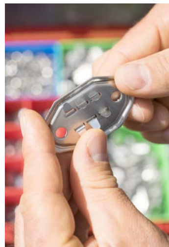
Third step: To fix the number inserts, bent them at the rear side (bending mechanism).
