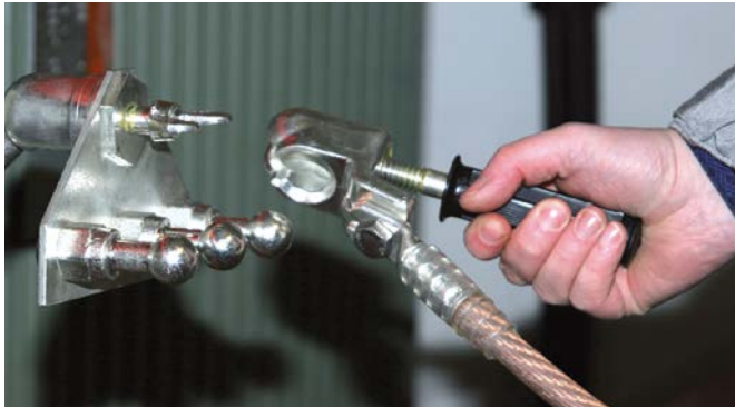
Earth connecting plate with fixed ball points and ball head cap with plastic handle.
