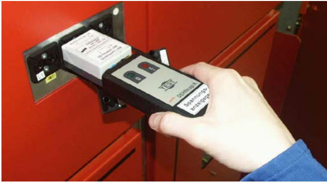
Self-test of a DEHNcap/A voltage indicator.
