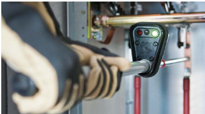
PHE voltage detector with visual indication.
