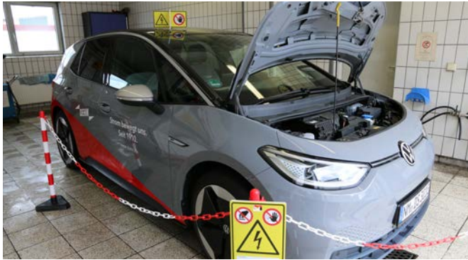
Clearly visible warning signs on the e-vehicle.
