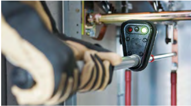
PHE voltage detector with visual indication.
