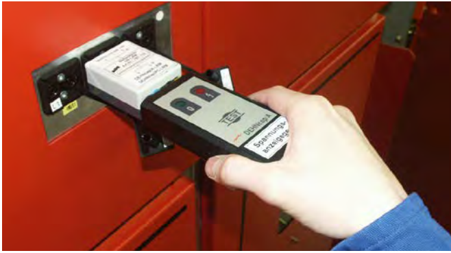
Self-test of a DEHNcap/A voltage indicator.
